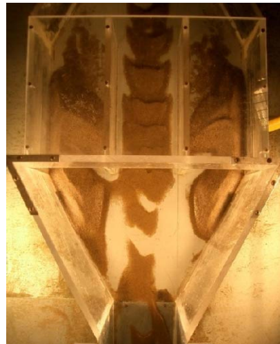
Figure 4-2-7 Sediment accumulation over 6 hours of observation
