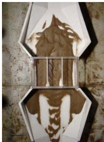
Figure 4-2-15 Hourly sediment accumulation in the expansion area for flow case B
