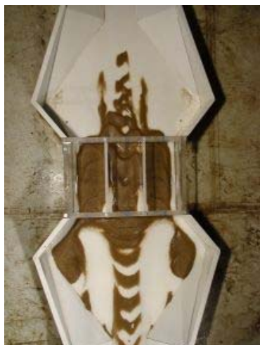
Figure 4-2-15 Hourly sediment accumulation in the expansion area for flow case B
