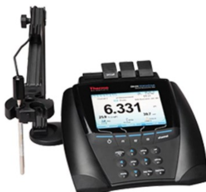
Figure 4.4. Benchtop Dissolved Oxygen Meter (Source: Thermo Fisher Scientific TM ).
